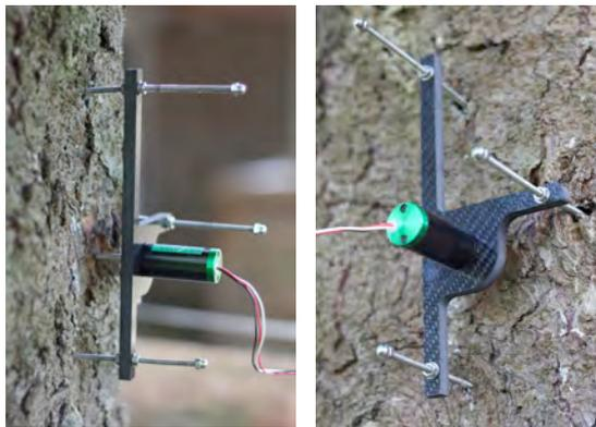
**Voltage-Sensitivity:** 1 mV = 4.0  $\mu\text{m}$
