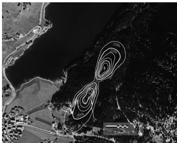
Fig. 1 Satellite image, location of flux tower (cross) and footprint area of Seehornwald Davos, Swiss Alps, computed with the footprint model of Kljun et al. (2004). The isolines show lines of equal relative footprint weights with respect to the point of maximum contribution during the time interval 1997–2004. The 20% and 50% relative contribution lines are drawn in bold. Background image © 2010 swisstopo (JD082776).
